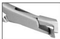
37-5077 Mini distal end cutters T.C with safety hold ● Max. 0.30 mm to 0.50 mm (.012" to .020") ■ Max. 0.46 mm to 0.64 mm (.018" to .025") ⊗ Max. 0.38 mm to 0.53 mm (.0155" to .0215") ⊗ Max. 0.53 mm to 0.64 mm (.021" to .025")
